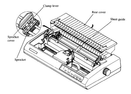
1 Remove the top and rear covers of the printer to insert the paper.
