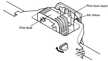
3 Use the grips on the side of the ribbon cartridge to help locate the cartridge (squeeze them inwards gently), and make sure that the spindles on the cartridge holder fit into the sockets on the cartridge itself.
