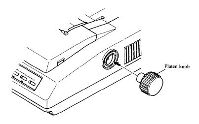
The platen knob should be removed from the accessory box inside the shipping carton. Mount the platen knob on the shaft on the right-hand side of the printer. Turn the knob on the shaft before pushing the knob fully into position.
