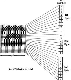
In the case of a superscript/subscript character, the width has also been defined by  $\langle al \rangle$ , but only two bytes are required per vertical column, so the arrangement is as follows: Bit
