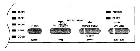
The principle involved is that the printer will print a list of options on one line. You use the  $(\underline{ser/\underline{RE}})$  and  $(\underline{rear})$  buttons to move the print head so that it is below the option you want to choose.
